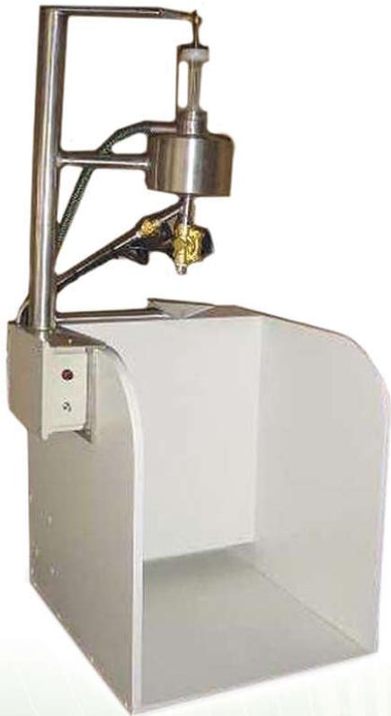
The water dispenser automatically dispenses the 2000g of water needed to be added to the cane sample, for homogenisation in the Cold Digester.
