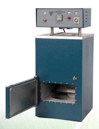
The Cane/Bagasse drying oven dries a sample of cane or bagasse in a stream of temperature controlled heated air at 105° C, for one hour in a pan with a nylon mesh base.
