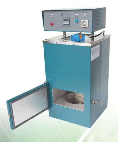
The Cane/Bagasse drying oven dries a sample of cane or bagasse in a stream of temperature controlled heated air at 105° C, for one hour in a pan with a nylon mesh base.
